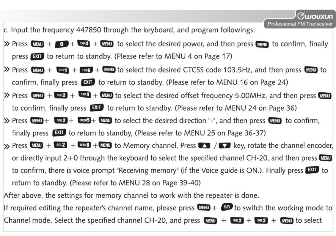
channel NAME displaying mode, press MENU to confirm, press EXIT to return to standby. Then press MENU + SOLZ + WOX7 + MENU to edit the channel name. After finishing editing, press MENU to confirm, then finally press EXIT to return to standby. (Please refer to MENU 22 on Page 33-35 and MENU 27 on Page 38-39)
